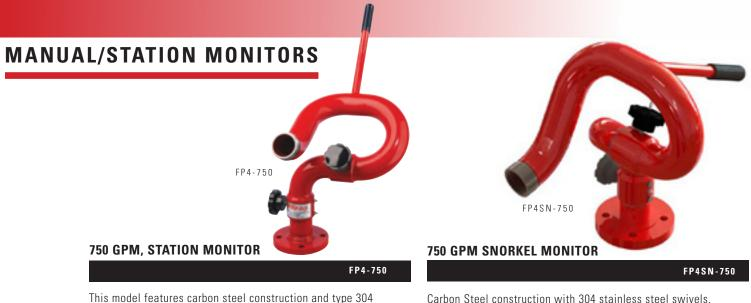
stainless steel swivels. Type 304 ball bearings in joints ensure easy movement and reliable operation. This monitor has a standard red polyester powder coating inside and out to protect against corrosion and offers 360° horizontal and 120° vertical travel.
