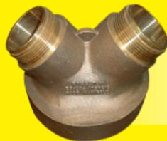
**A ROOF CONNECTION** is used as a standpipe roof outlet connection by the fire service. It provided the NFPA-14 required 250 GPM per outlet. Angle or straight values are normally supplied with the connection.
